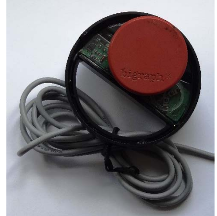
Figure 5. Briefly place magnet near reed switch
